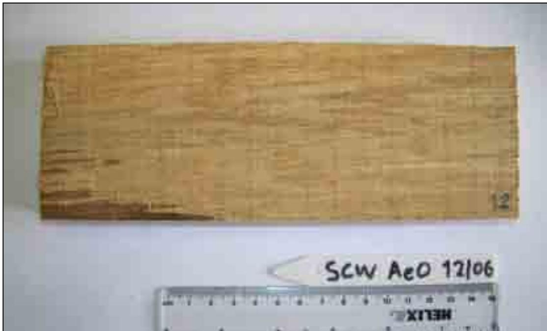
**Figure 6 Sacrificial sample before deployment**
