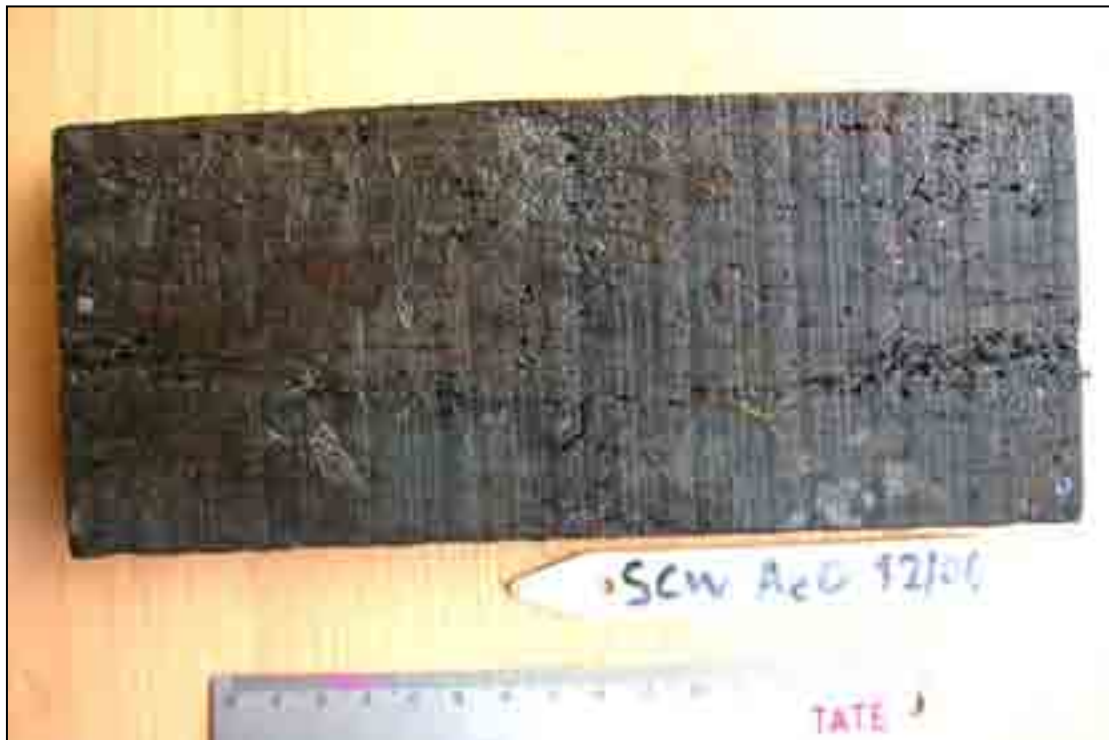
Figure 7 Same sacrificial sample as before after 3 months deployment
