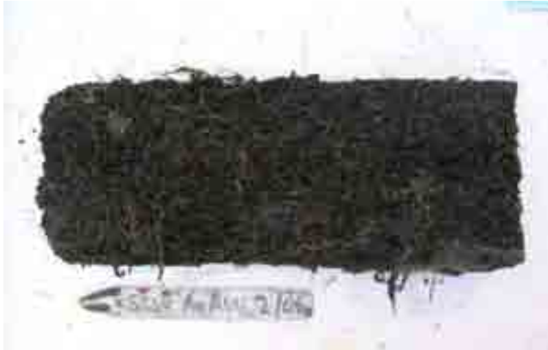
Figure 3 Sample deployed for 12 months - shows complete surface degradation, grade 3
