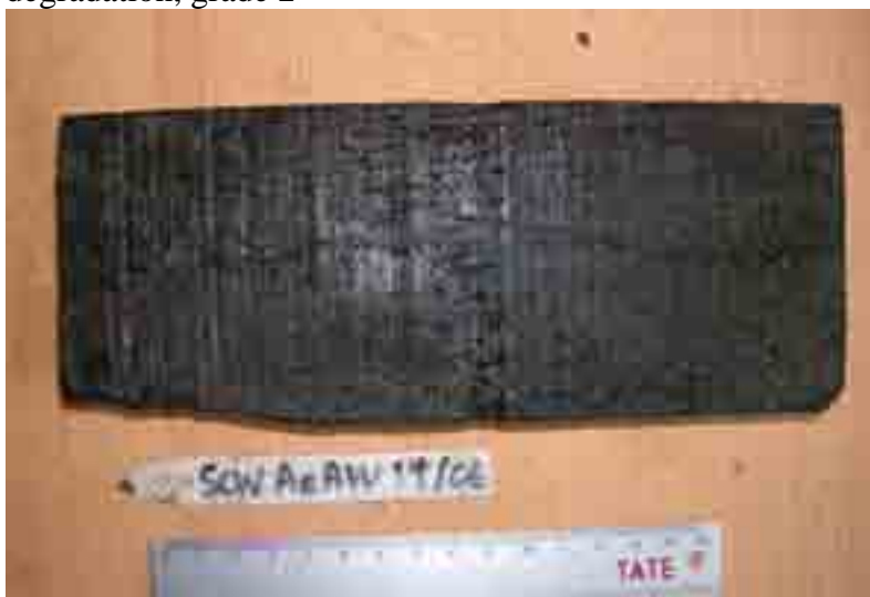
Figure 5 Sample after 3 months deployment - shows slight surface degradation, grade 1
