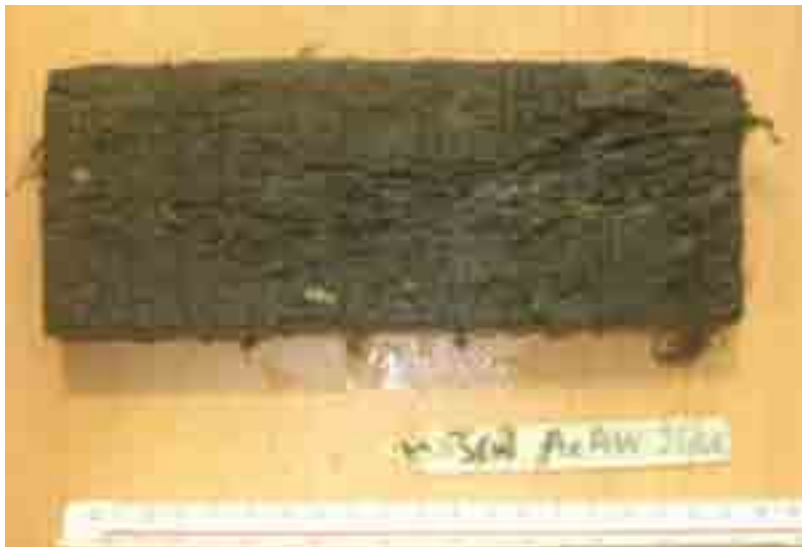
Figure 4 Sample after 6 months deployment - shows moderate to severe surface degradation, grade 2
